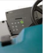
Optional 1-Step™ start button simplifes operator training with controls that enable sweeping systems to be activated with a single green button
