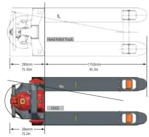
Y The short body length of truck (L2=380mm) is even smaller than Hand Pallet Truck. it provides the shortest turning radius of 1274 / 1336 mm with lifted/lowered forks and makes the truck extremely compact and ideal for use in confined spaces of retail stores, elevators or business centers.
