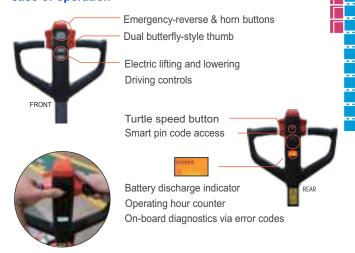
Y The function of driving with tiller in the vertical position helps with operations in confined areas without sacrificing safety
