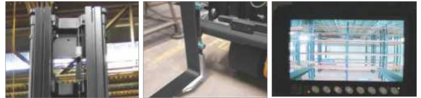
1. Mast / fork mounted camera and colour monitor
