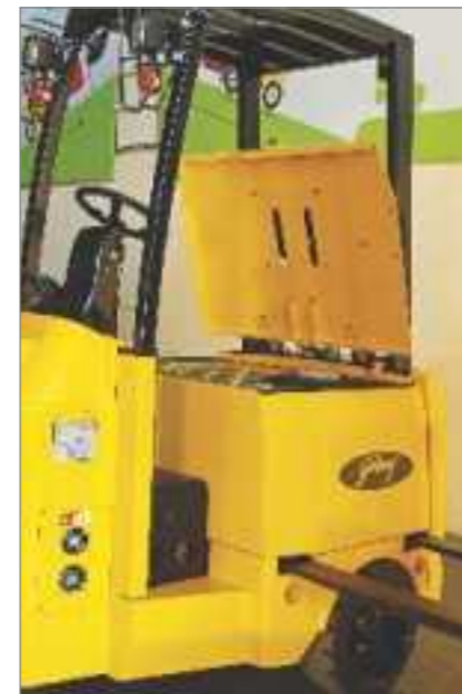
Fork pockets for easy removal of battery
